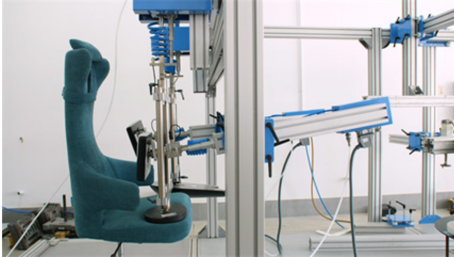
Figure 5.2.14 Office chair being mechanically tested
